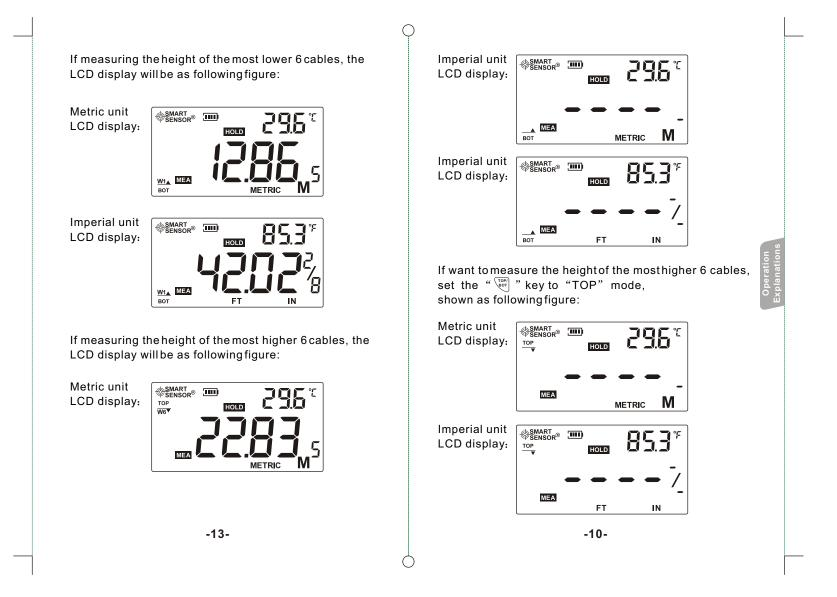
5). Hold level and steady the unit with two hands before chest part, press the " <sup>with</sup>" key for 1~2 seconds the LCD will show the symbol "HOLD", you can measure totally 6 cables height at one time, and measured data and such as W1、W2、W3、W4、W5、W6. Press the "SELECT" key you will read the measured data from W1 to W6 in turn, shown as following figure:
